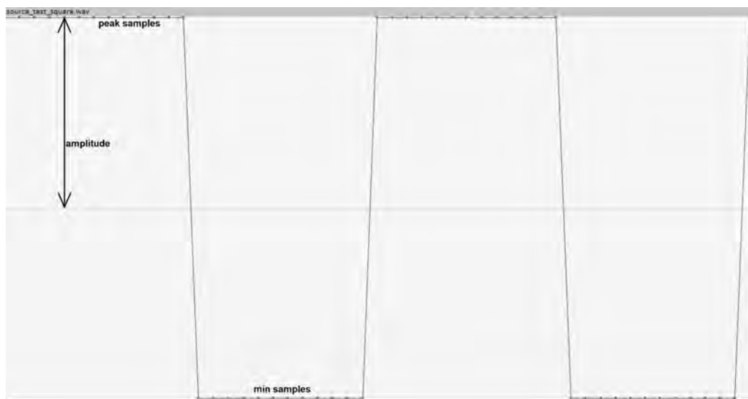
Figure 4.10: Properties of a square wave
