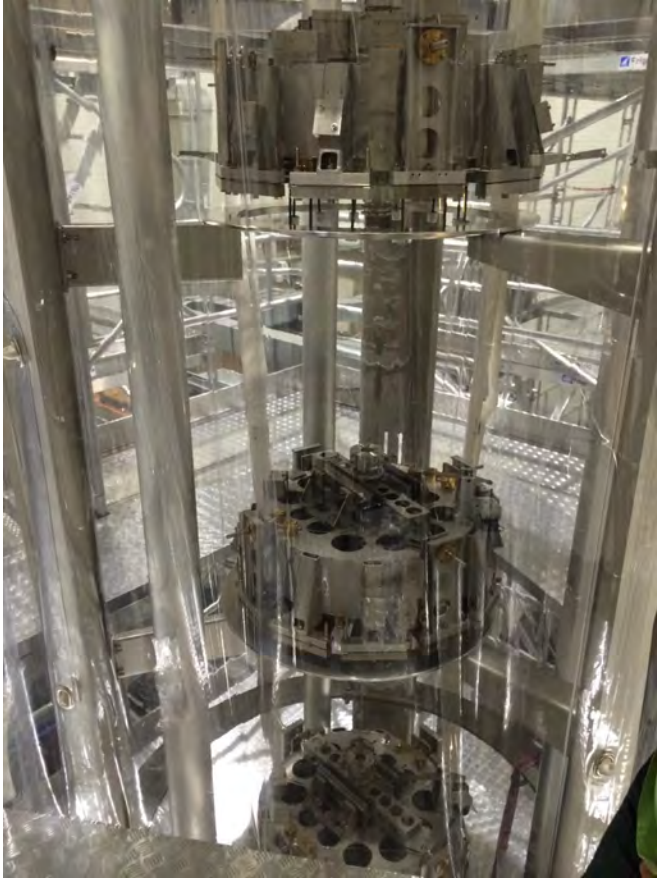
Figure 5.6: A portion of the Virgo detector's 8 m multi-stage pendulum from which the mirror is suspended. Photo courtesy: EGO/Virgo [162].
