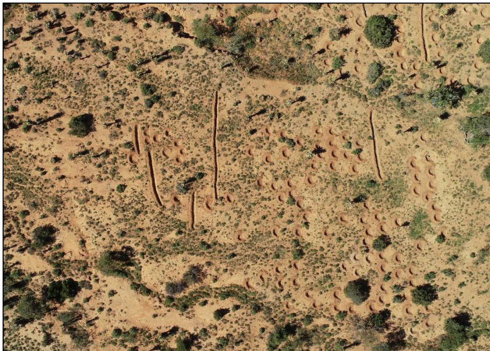
Fig. 1.17 Large-scale ecosystem restoration efforts in the Baviaanskloof, featuring soil degradation mitigation measures such as ponding and energy breaks, which are visible in this aerial image (Photo credit: Living Lands, 2019).
